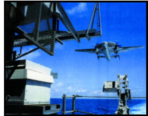
E-2C Hawkeye landing aboard CV-64. (The Laser Centerline Localizer Long-Range Line-up System is visible as the gray box on the left hand side.)
