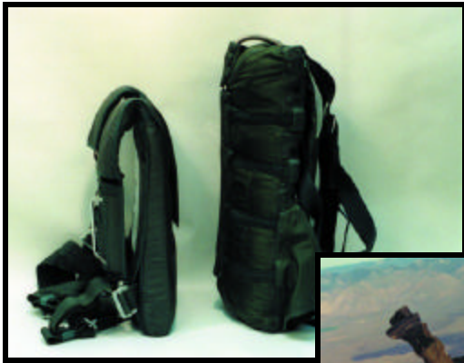
SEI's Durachute Thinpack emergency bailout parachute (left), compared to the old NB-8 parachute of the U.S. Navy (right)
