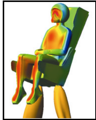
Modeling the effect of rocket plumes on ejection seat aerodynamics
