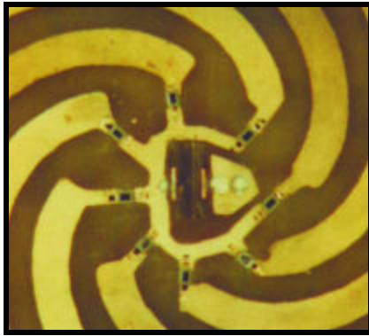
Exploded view of feed region of the SMM antenna/phase-shifter showing PIN diode switches
