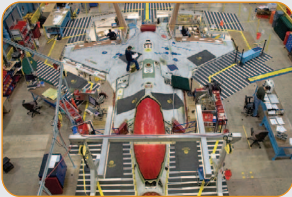
An overhead view of F-35A-1 shows the canopy and rear of the plane just installed. Photo courtesy of Lockheed Martin.
