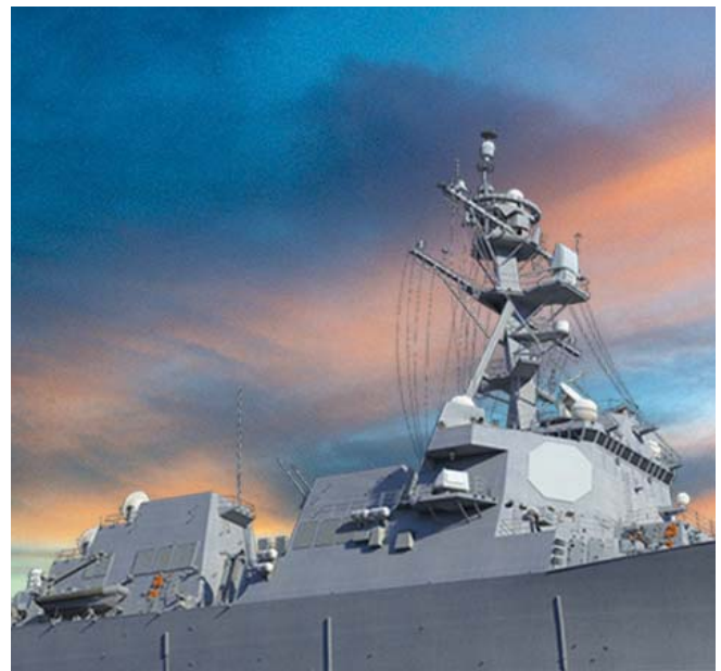
This illustration shows a U.S. Navy destroyer equipped with the new Air and Missile Defense Radar. The groundbreaking Raytheon-built system's electronics will provide 30 times the sensitivity of the radar on board today's destroyer fleet. (Raytheon)
