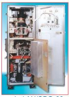
Upgraded AN/SPG-60 Radar Transmitter
