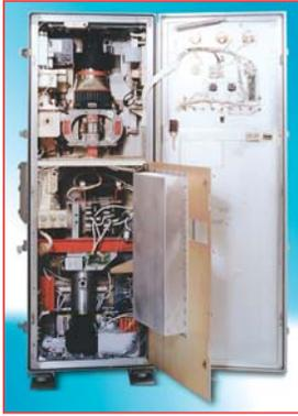
Upgraded AN/SPG-60 Radar Transmitter
