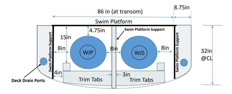
Deck of swim platform is 33 in Fore/Aft and 60 in wide at furthest aft point
