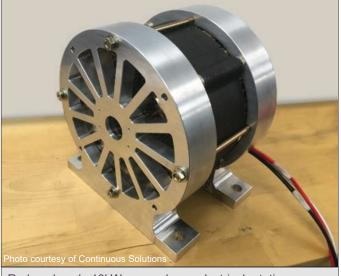
Reduced-scale 10kW power-dense electrical rotating machine built by Continuous Solutions
