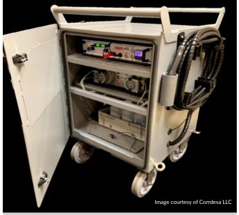
Corrdesa partnered with DALIC to produce the ruggedized mobile Dalistick® system for ZnNi plating repairs directly on aircraft.
