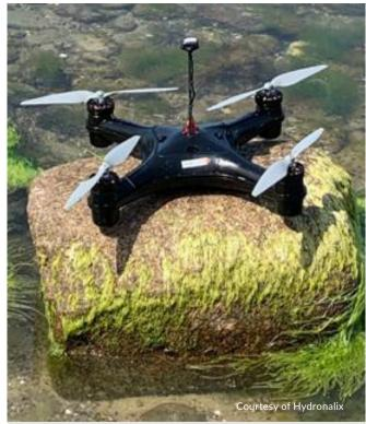
The ADAPT disposable drone can deliver a payload to an exact location up to a mile and a half away.
